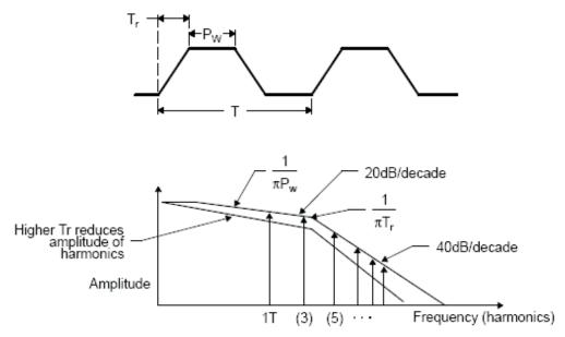
Figure 2. Time Domain and Frequency Domain of a Clock Signal
