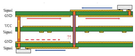
Figure 14. Loop Areas Caused by Poor Via Placement
