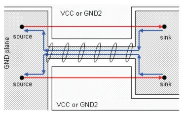
Figure 10. Crosstalk Induced by the Return Current Path
