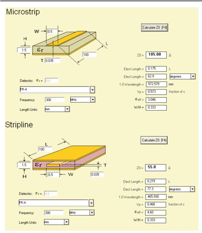
Figure 4. Calculation of Properties of Microstrip and Stripline (AppCAD)
