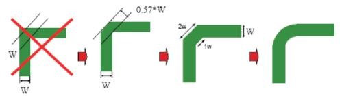
Figure 13. Poor and Good Right Angle Bends
