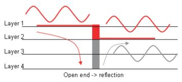
Figure 16. Reflection Caused by Stubs in a Via
