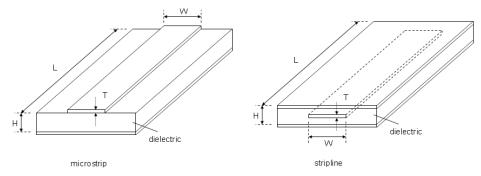
Figure 3. Structure and Dimension of Microstrip and Stripline
